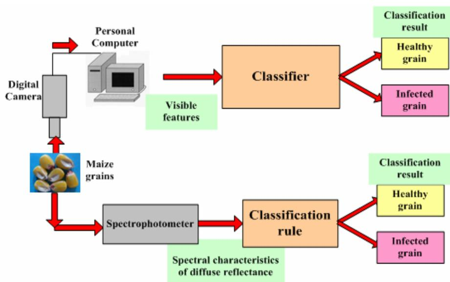
Fig. 1 Main steps in both methods – near infrared spectroscopy and analysis of the images
