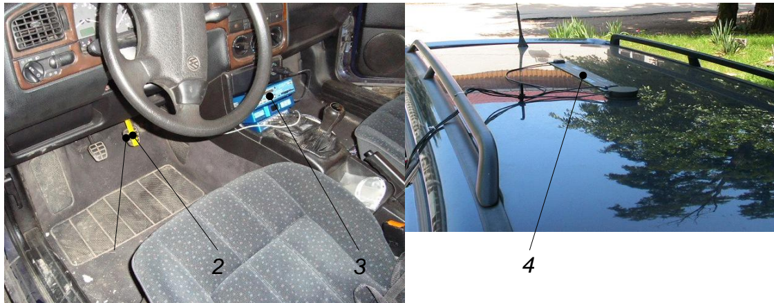
Fig. 4. Equipment of the test car: 1 - Brake pedal; 2 - Brake trigger; 3 - VBOX 3i logger; 3 - GPS antenna
