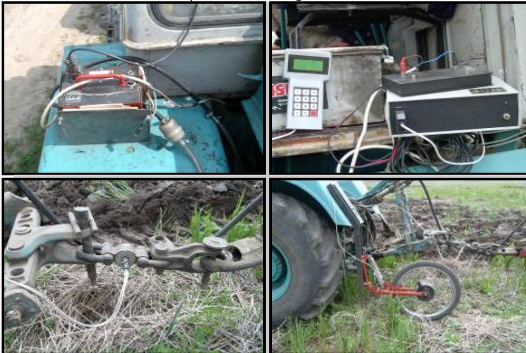
Figure 2. Parts of the ASIT-1 microcomputer system used for experimental testing of tractors and automobiles
